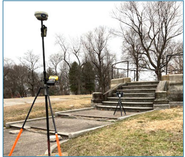
Frontenac Engineering made 3D laser scans and topographic survey of bandstand ruins and surrounding area.
